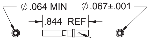
16 GAUGE CONTACT DETAIL \phi .039 INSPECTION HOLE
