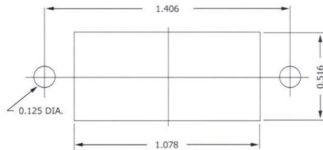
RECOMMENDED CHASSIS CUT-OUT
