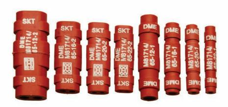
DME In-Line Junctions provide environment resistant performance in either two wire or bussed four wire configurations. Both types use standard MIL-39029/22 socket contacts. All DME Series In-Line Junctions are qualified to MIL-T-81714E (Series II)\* and are completely interchangeable with the Deutsch CTL/ CTM In-Line Junctions.
