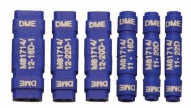
Built and qualified to MIL-T-81714E, DME wire splices provide a reliable positive and maintainable connection for two and four wire applications. All use the standard M39029/1 pin contact. The new D environmental class splice supersedes part numbers of the preceding A, B, and C environmental classes thus eliminating the cumbersome multiple environmental class system.
