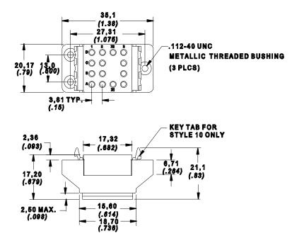
For use with E405 and ES405 Relays with Mounting Code 2 (Adapter Kit required) or G and Pin Code M
