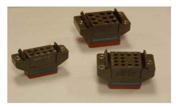
The SLDE Snap Lock series sockets are compatible with DRI "E" series 2 and 4 pole 5 Amp relays, 2, 3, and 4 pole 10 / 15 Amp relays, and 3 pole 25 Amp relays conforming to MIL-PRF-83536. We have engineered these sockets to allow for easy one sided access with no loose parts, saving on installation and replacement time, and significantly reducing if not eliminating the chance for FOD to develop. These sockets are for use with captive screw type relays, or for use with the available adapter kit.
