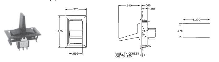
1 Three and four pole switches require assembly from back of panel.
