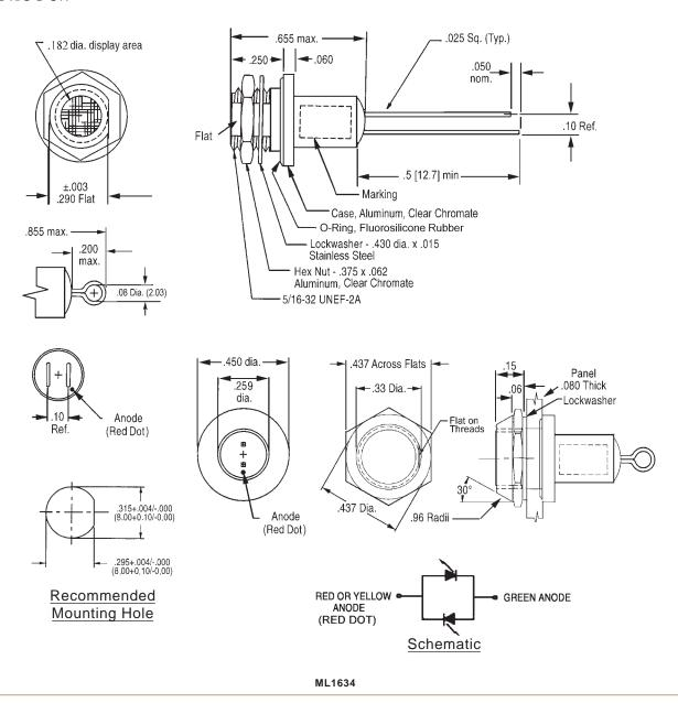
NOTE: Dimensions in ( ) are mm. Tolerances: Decimals: ± .010 (0.25) Fractions: ± 1/64 Mounting Torque: 5-7 in. lbs.
