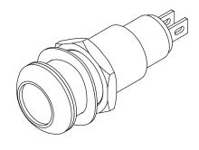
ML 5116 Panel Indicators are rugged durable LED indicators that are suitable for mounting. These indicators are IP67 sealed for external functionality and feature internal potting for vibration control and durability to withstand industrial applications. Indicators meet specific military specifications listed in data sheet. These indicators come in a variety of colors and with AC or low voltage applications. Refer to the product specifications for additional details.
