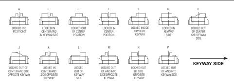
Figures A thru P do not represent details of construction. They schematically illustrate locking function.
