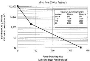
\*Failure mode: Dielectric withstand voltage test @ 2000 Vdc, power terminal to terminal, leakage exceeds 1.0 A. Current Carry: 500 A @ 25°C. Derate 2.5
