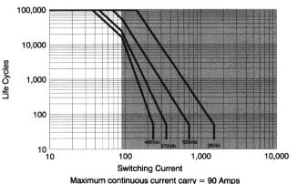
\*Based on data extrapolated from qualification at 270 Vdc with resistive load. Since each application is unique, user is encouraged to verify rating in actual application.
