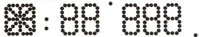
Front View Front View Front View Front View Front View Front View 16 Segment Colon 2-7 Segment Degree 3-7 Segment Decimal Point A6 A15 A11 A16 A12 A14
