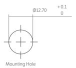
Anode termination indicated by red sleeve. Mounting hole to be clean and burr free.
