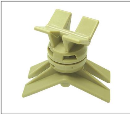
Amphenol Pcd's Cable Separators are used to help separate cable harnesses from one another, aiding in organizing cable routing throughout the aircraft. Available in either Nylon or PEEK, they maintain clearance between two parallel or crossing cable harnesses preventing wire abrasion. Nine different versions are available and they are qualified to Airbus standard ABS1144.
