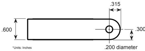
Engineered for lean manufacturing, the high performance P-Clamps were developed to replace and out perform traditional P-Clamps and Saddle Clamps. Featuring an overmold silicone cushion with PEEK polymer, our clamps are completely non-conductive/non-corrosive, lightweight, and very durable.
