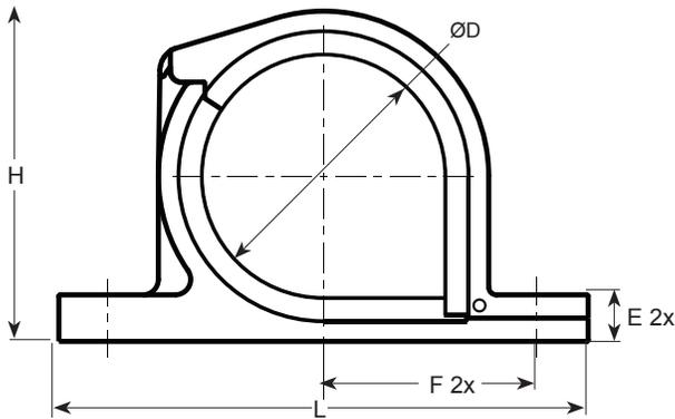
Engineered for lean manufacturing, the high performance Omega Clamps were developed to replace and out perform traditional P-Clamps and Saddle Clamps. Featuring an overmold silicone cushion with PEEK polymer, our clamps are completely non-conductive/non-corrosive, lightweight, and very durable.
