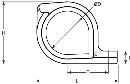
Amphenol Pcd's LDG P-Clamps use a soft rubber for clamp cushioning, thereby reducing wear and tear on mission-critical cable harnesses without compromising the strength and performance of the clamp itself. Specifically designed for high performance aerospace cables, such as the MT/MTL product lines, they are easy to use, simple to maintain, and available in 17 different sizes.
