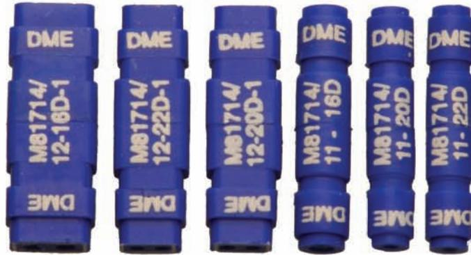
Built and qualified to MIL-T-81714E, DME wire splices provide a reliable positive and maintainable connection for two and four wire applications. All use the standard M39029/1 pin contact. The new D environmental class splice supersedes part numbers of the preceding A, B, and C environmental classes thus eliminating the cumbersome multiple environmental class system.
